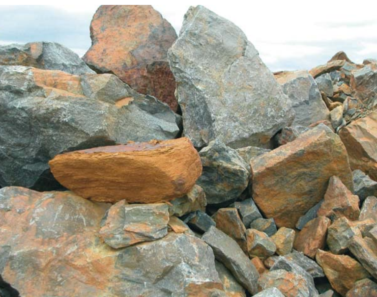
Figure 37. Waste rock generated during mining varies greatly, from dust and sand-sized particles through to large boulders.
