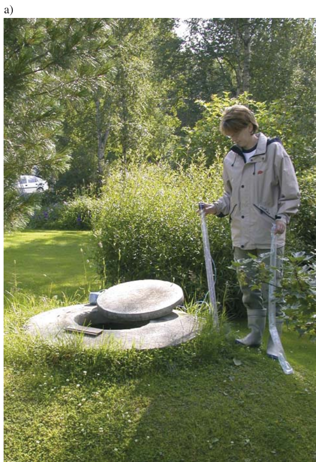
Figure 48. Groundwater samples for monitoring purposes can be taken from (a) existing domestic wells, or (b) from observation wells.
