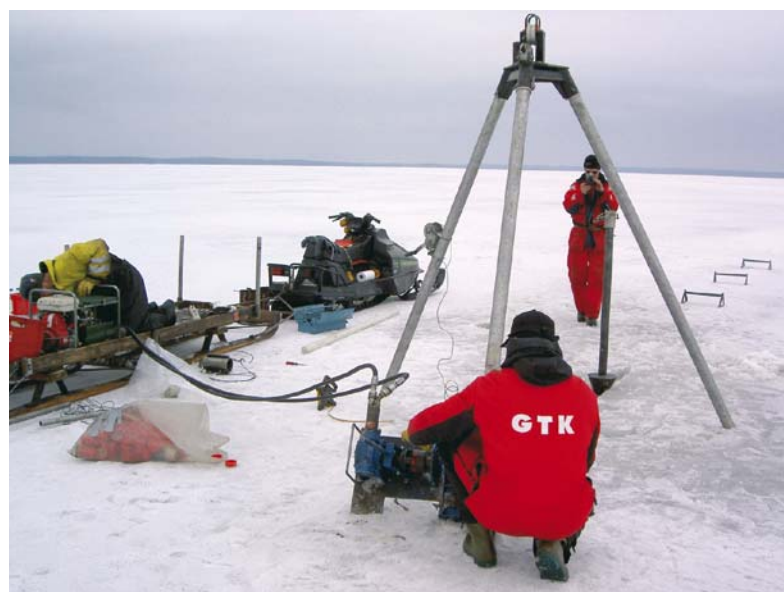
Figure 25. Portable drilling equipment transported by snowmobile is capable of retrieving sediment cores up to several meters in length, enabling assessment of the effect of mining activities on sediment and pore water composition, and characterization of environmental parameters prior to mining.
