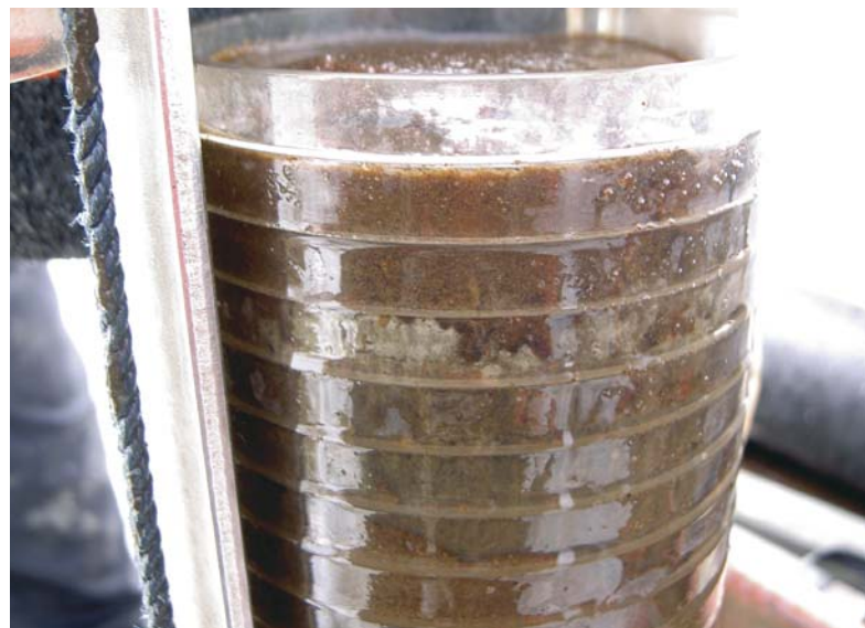
Figure 24. The extent to which mining activities influence water quality in streams and lakes subject to mine water discharge can be evaluated by analysis of contaminant abundances in recent sediments. Use of a Limnos sampler enables retrieval of undisturbed samples.
